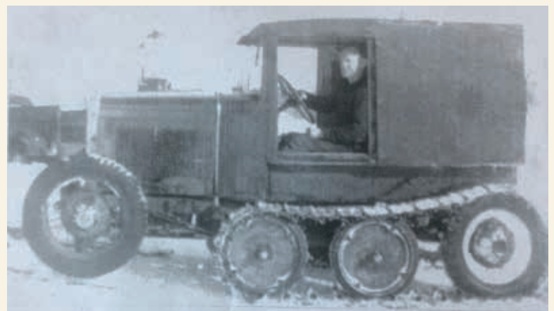
George Thompson, relief mail carrier, created a truck "snowmobile" with skis in front and tracks in the back.
